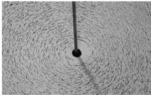
Fig. 29-3 Iron filings that have been sprinkled onto cardboard collect in concentric circles when current is sent through the central wire. The alignment, which is along magnetic field lines, is caused by the magnetic field produced by the current. (Courtesy Education Development Center)
